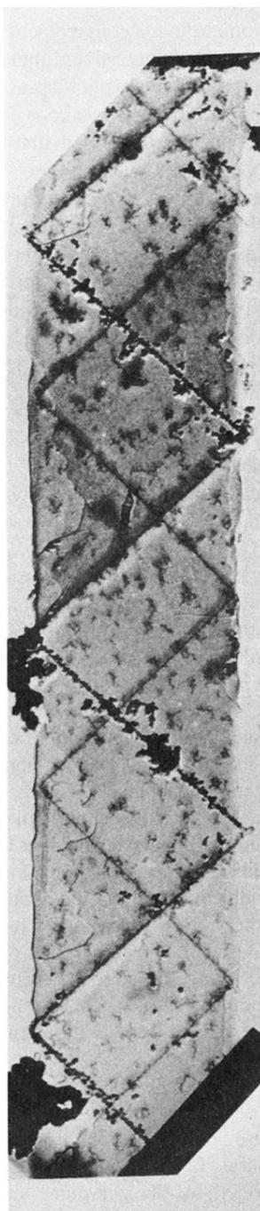
FIG. 1. Transmission electron micrograph of a tubule with adsorbed Pd-Ni catalyst particles on the surface [4]. The diameter of the tubule is approximately 0.5 \mu\text{m} . Reprinted from Ref. [19].
