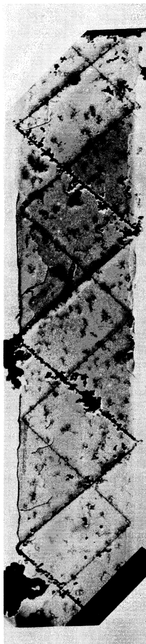
FIG. 1. Transmission electron micrograph of a tubule with adsorbed Pd-Ni catalyst particles on the surface [4]. The diameter of the tubule is approximately 0.5 \mu\text{m} . Reprinted from Ref. [19].
