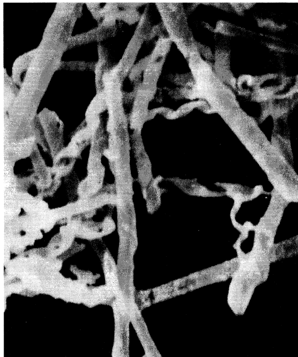
FIG. 2. Scanning electron micrograph of helical ribbons formed from a racemic mixture of D and L diacetylenic phospholipids. Note that the racemic mixture forms distinct right- and left-handed helical ribbons. The diameter of the helical ribbons is approximately 0.5 \mu\text{m} . Reprinted from Ref. [9] with permission (© 1988 Elsevier Scientific Publishers).
